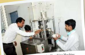
Ten Station Rotary Tablet Punching Machine with B and D Toolings (Aidmach)
