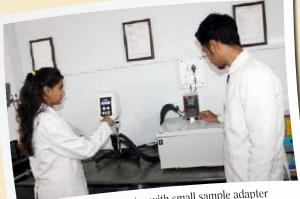
Brookfield Viscometer with small sample adapter (Ametek, DVE Viscometer)
