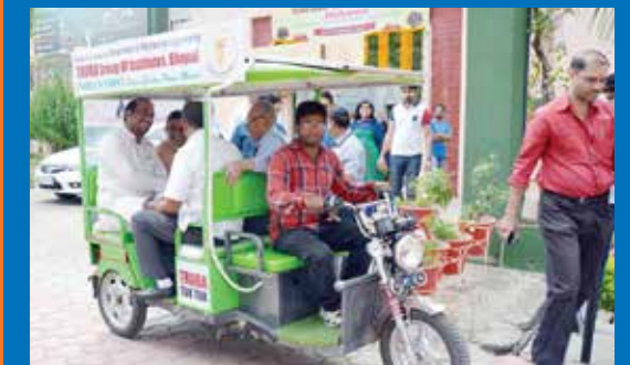
Students of BE-Mechanical VIII semester developed a Solar Hybrid Three wheeler, Truba Tuk Tuk.
